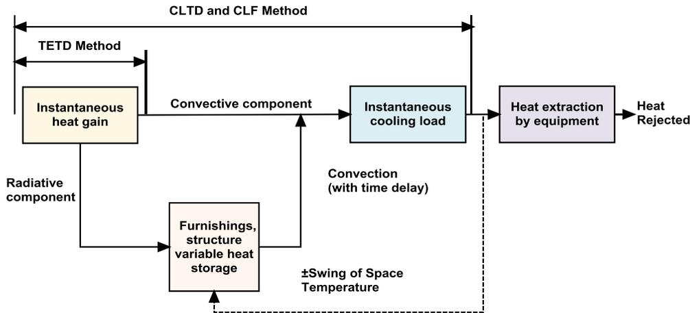
Figure 1. Schematic of Load Transfer [1]
