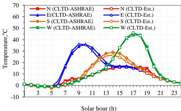
Figure 5. Comparison of CLTD values estimated by CFFT and given in ASHRAE 1997 [17] for Wall 1 due to main directions.
