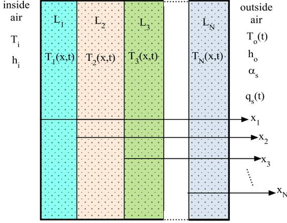
Figure 2. A schematic representation of a multi-layered wall
